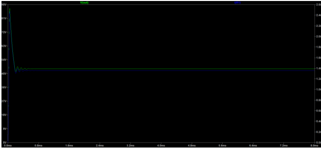
Fig. 8. Load voltage and current measurement for input voltage of 150V, load resistance of 35 \Omega and duty cycle of 0.32
