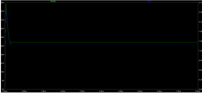
Fig. 7. Load voltage and current measurement for input voltage of 210V, load resistance of 35 \Omega and duty cycle 0.23
