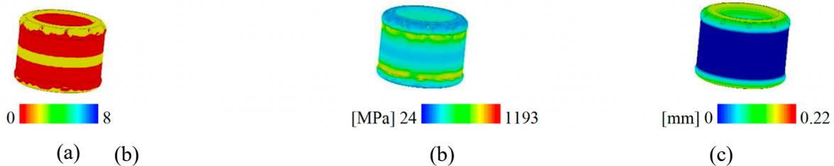
Fig.6. Can Simulation results for: (a) Safety Factor (Per Body). (b) Von Mises. (c) Displacement
