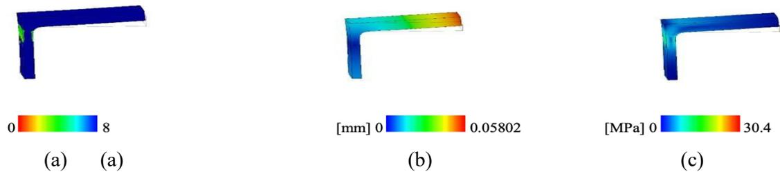
Fig.5. Handle simulation results for: (a) Safety factor (Per Body). (b) Displacement. (c) Von Mises
