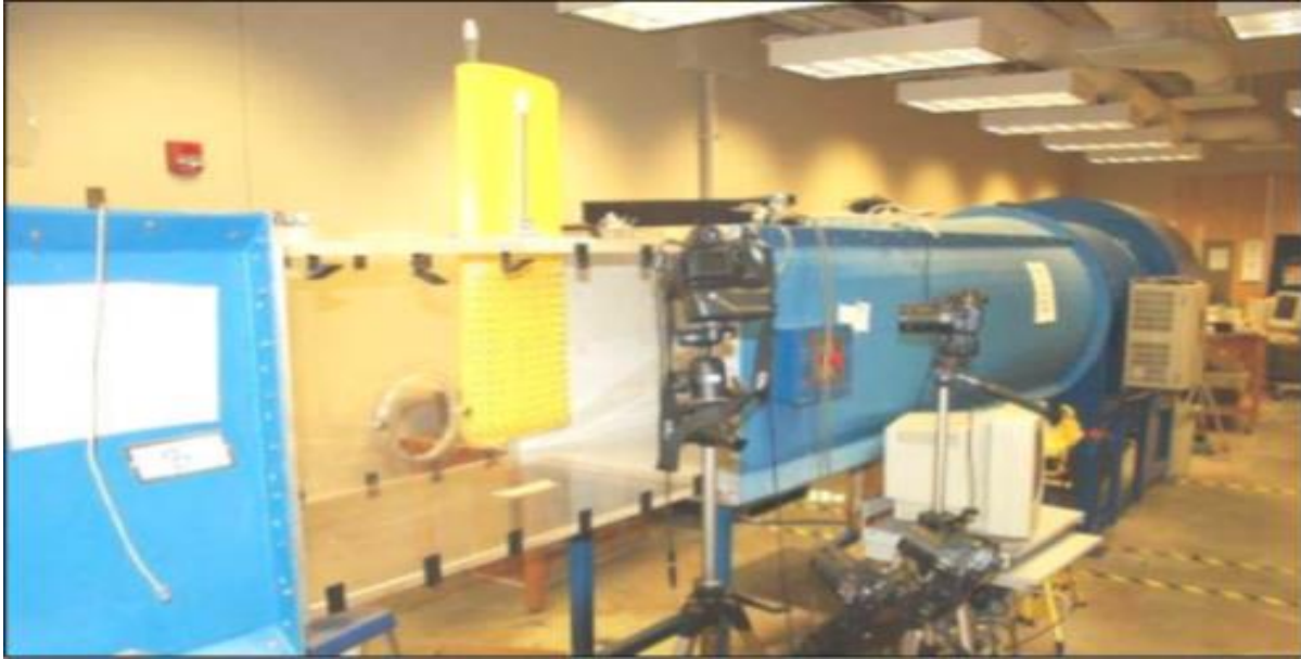
Figure 1: Inflatable wing in a wind tunnel with fiducial markers at the University of Kentucky.
