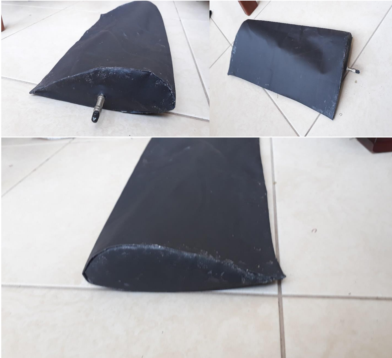
Figure 6. Finished inflatable wing prototype
