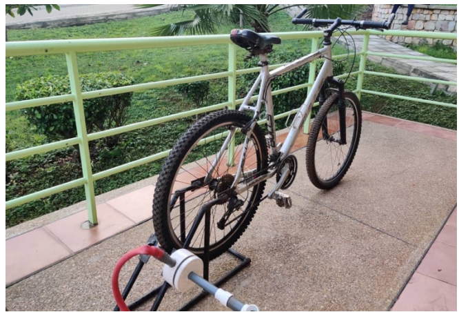
Fig.11b – Complete bike water pump
