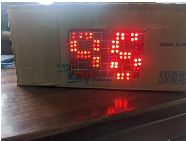
Figure 9: Final Product, With the sensors and LED enclosed in a box (showing an object count of 95)
