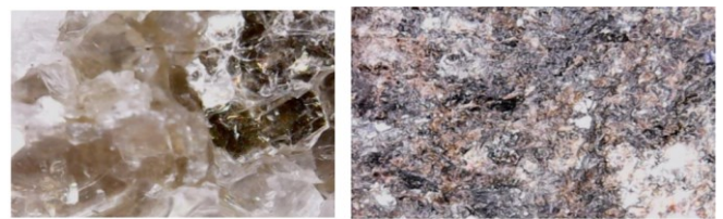
Figure 4: USB microscopic shots of the cassiterite and sphalerite ores on the left and right sides respectively
