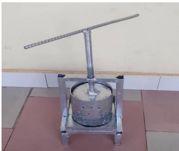
Figure 6: (a) Prototype of the torsional compression thread-based gari screw-type press (cassava pulp mechanical dewatering machine)
