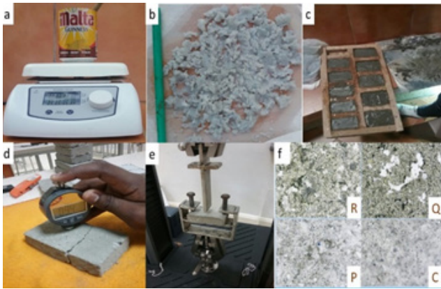
Figure 1. Procedure (a) Melting of plastics, (b) Drying of the plastic granules, (c) Molding of blocks, (d) Testing Hardness, (e) Microscopic surface analysis of different samples
