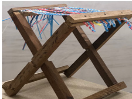
Fig.5. Resulting foldable wooden stool with seating area made out of plastic straw woven in a rustic plait.
