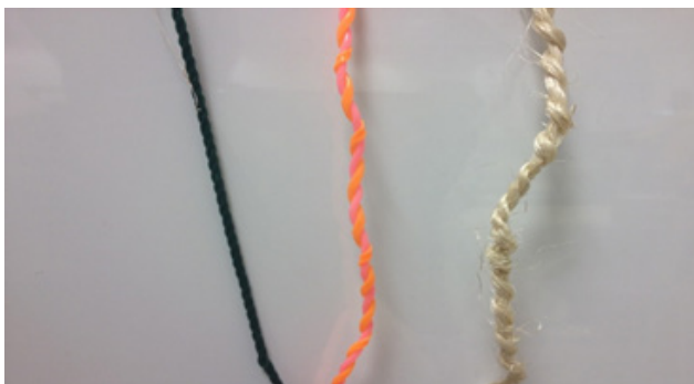
Figure 1. A picture of the three samples: nylon(deep green), rubber(orange), and sisal white).
