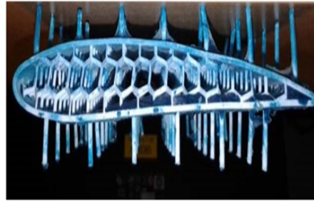
Figure 2. (a) The lattice structure wing. (b) Hexagonal diamond structure of the inflatable wing
